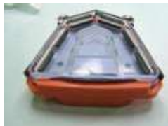
Place the tray on the silicone former
