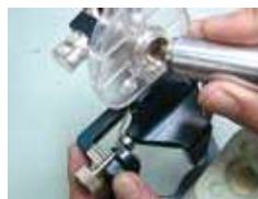
Use magnet removal bar take out of the magnet on the upper mounting plate
