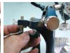
Set the pin to make sure the upper frame is parallel to the lower frame
